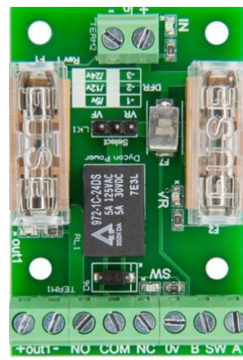
DFR-1-12 (12VDC unit) or DFR-1-24, (24VDC unit) relay board that switches the output power if the input is closed or opened.
